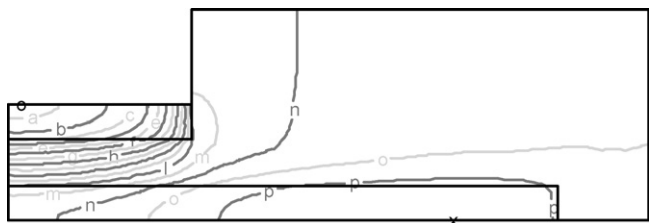
Fig. 5. Simulation of electrolyte potential distribution near edge of a lithium-ion cell (see Fig. 3) with negative electrode extending 0.4 mm past the positive at 10 s into a 5 C discharge pulse at 60% SOC. Lettered isopotential lines are shown at about 5 mV intervals.
