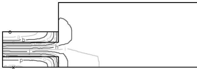
Fig. 4. Simulation of electrolyte potential distribution near edge of a lithium-ion cell (see Fig. 3) with electrodes aligned at 10 s into a 5 C discharge pulse at 60% SOC. Lettered isopotential lines are shown at about 4 mV intervals.
